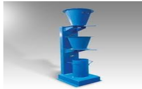
Fig no: 4.1 - Compaction factor test apparatus
