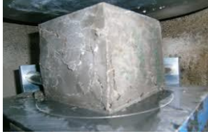
Fig no: 4.2-Concrete Cube testing
